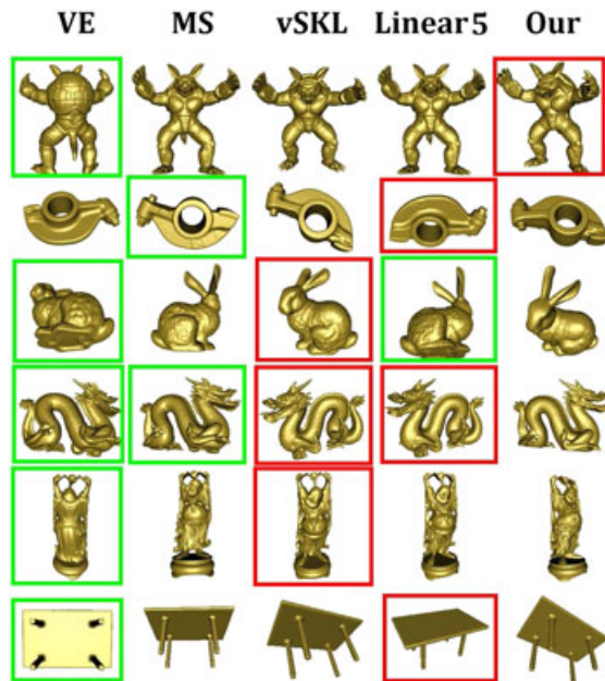
Figure 3. The good views of some tested models obtained with the methods in comparison. Here, the views with the highest and lowest averaged rank scores are marked in red and green boxes, respectively.
